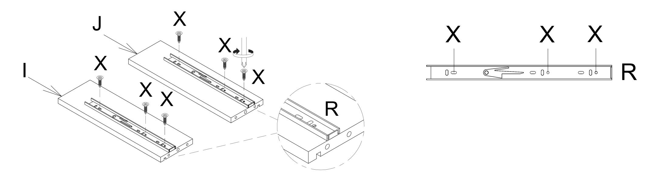
Attach Dowel (S) and Cam Lock (V) to the Left & Right Small Drawer Side (I & J) and the Small Drawer Back (L). Attach Cam Bolt (U) to the Left & Right Small Drawer Side (I & J) and the Small Drawer Front (K) with a screwdriver (not provided).
