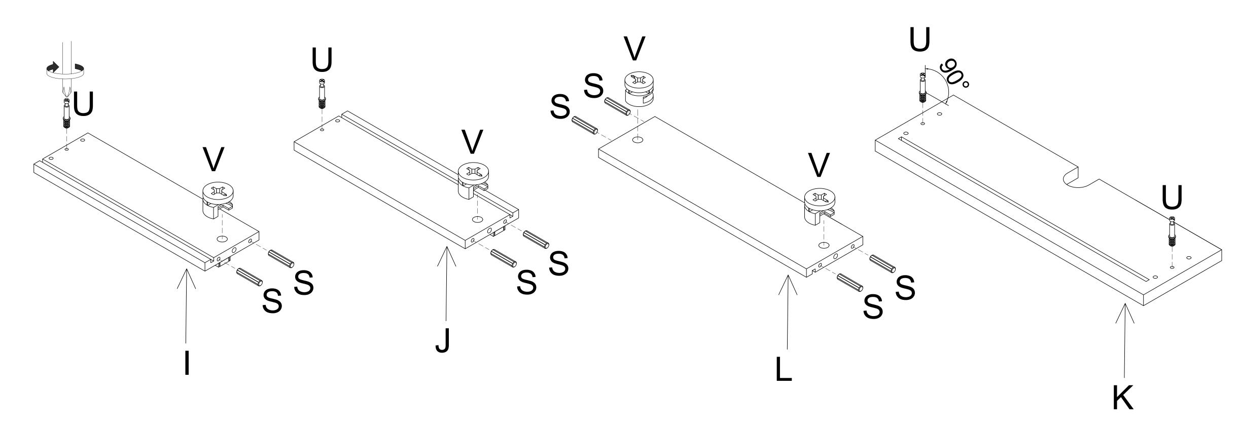
Attach the Left & Right Small Drawer Side (I & J) to the Small Drawer Back (L) and secure the Cam Lock (V) with a screwdriver (not provided). Cover the Cam Lock (V) with Cam Lock Cover (W).
