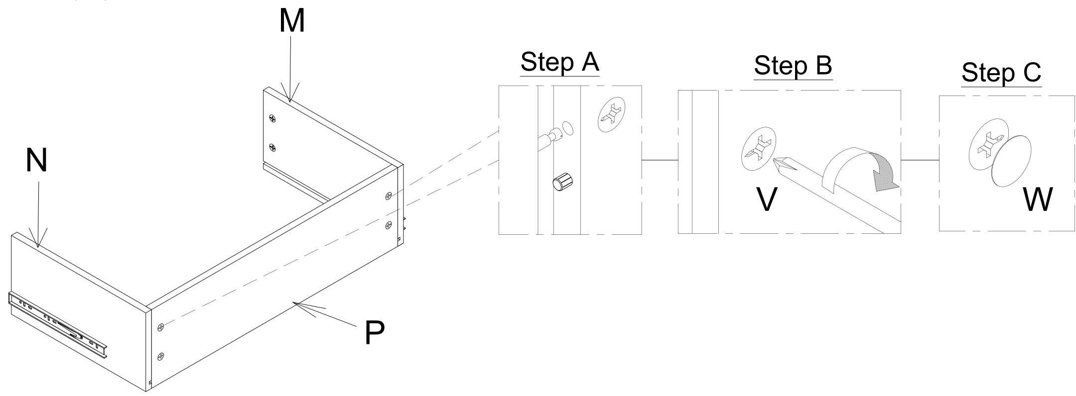
Slot the Drawer Base (Q) into the grooves of the drawer box. Attach the Big Drawer Front (O) to the drawer box and secure the Cam Lock (V) with a screwdriver (not provided). Cover the Cam Lock (V) with Cam Lock Cover (W).
