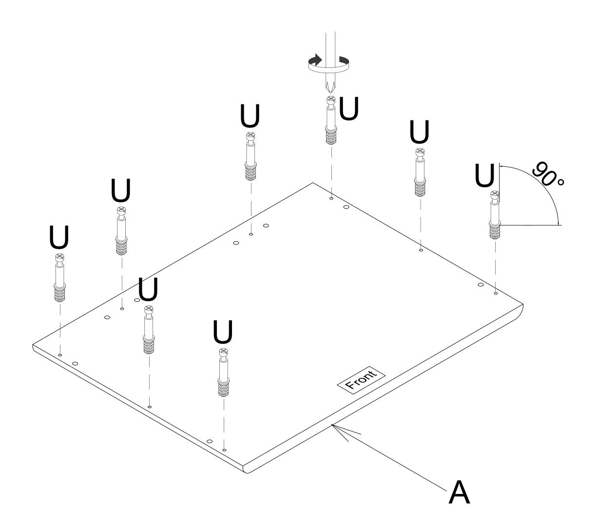
2 Insert Dowel (T), Cam Bolt (U) and Cam Lock (V) into the Left & Right Side Panel (B & C) with a screwdriver (not provided).
