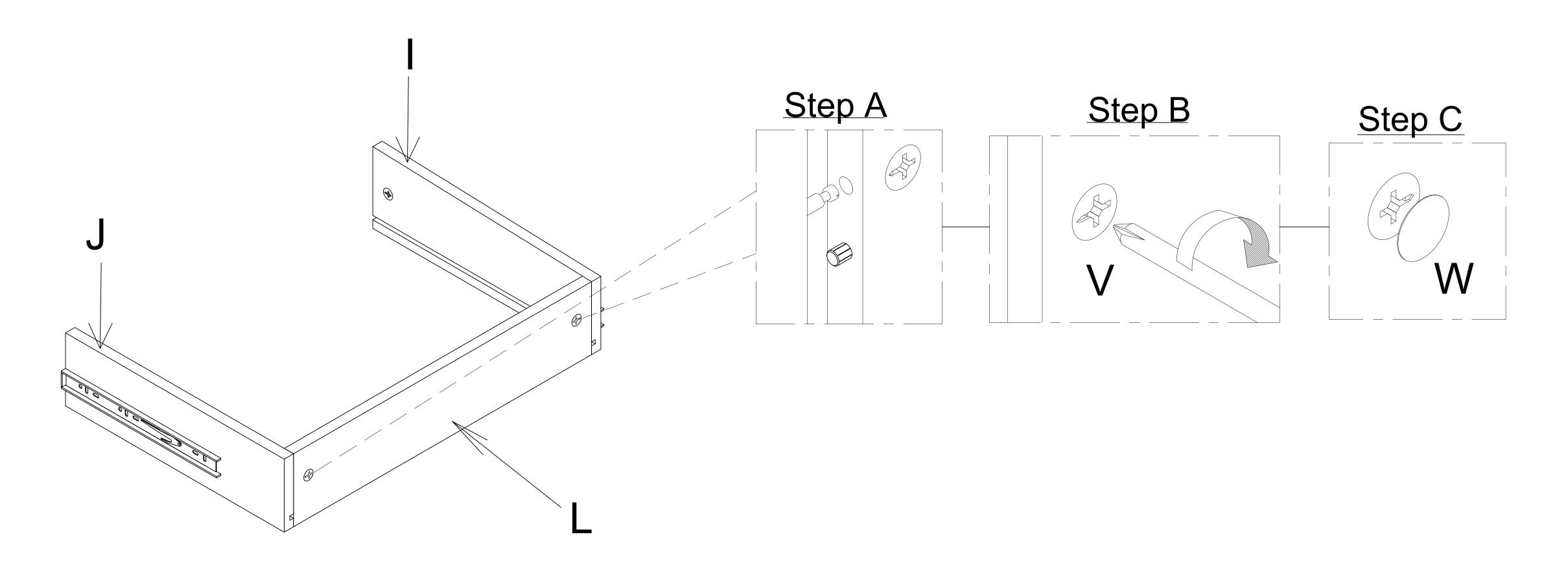
Slot the Drawer Base (Q) into the grooves of the drawer box. Attach the Small Drawer Front (K) to the drawer box and secure the Cam Lock (V) with a screwdriver (not provided). Cover the Cam Lock (V) with Cam Lock Cover (W).
