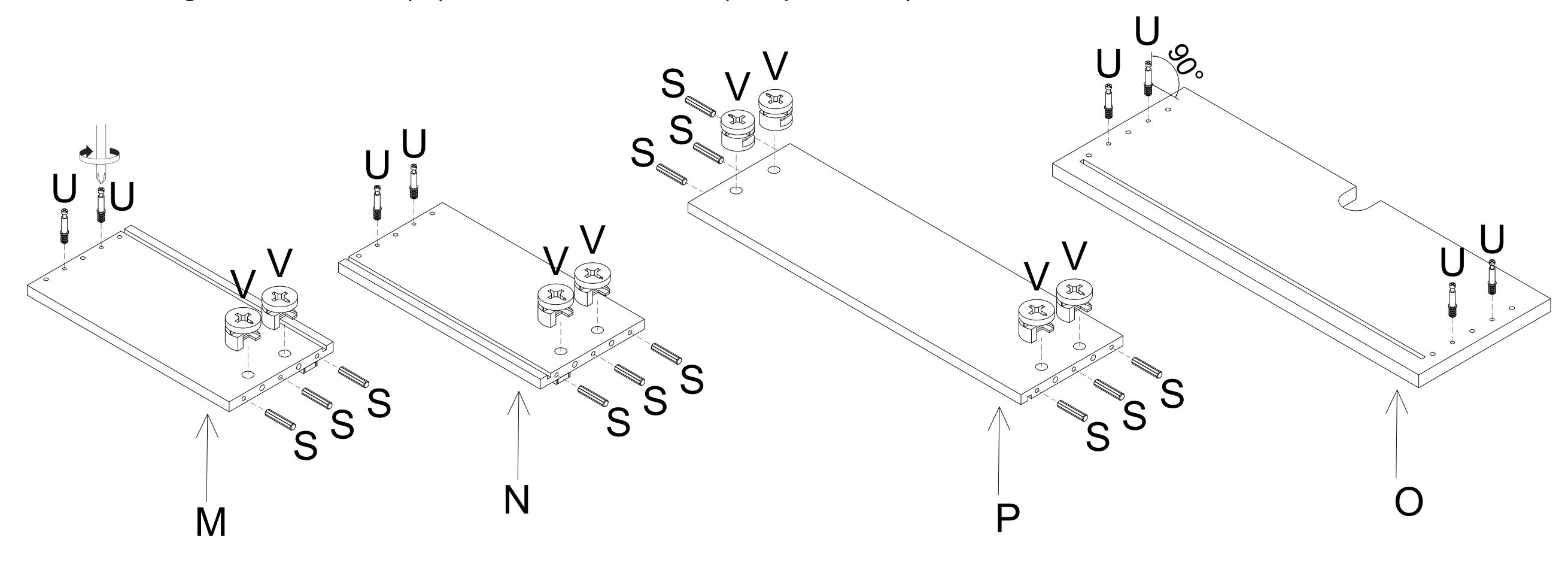
Attach the Left & Right Big Drawer Side (M & N) to the Big Drawer Back (P) and secure the Cam Lock (V) with a screwdriver (not provided). Cover the Cam Lock (V) with Cam Lock Cover (W).
