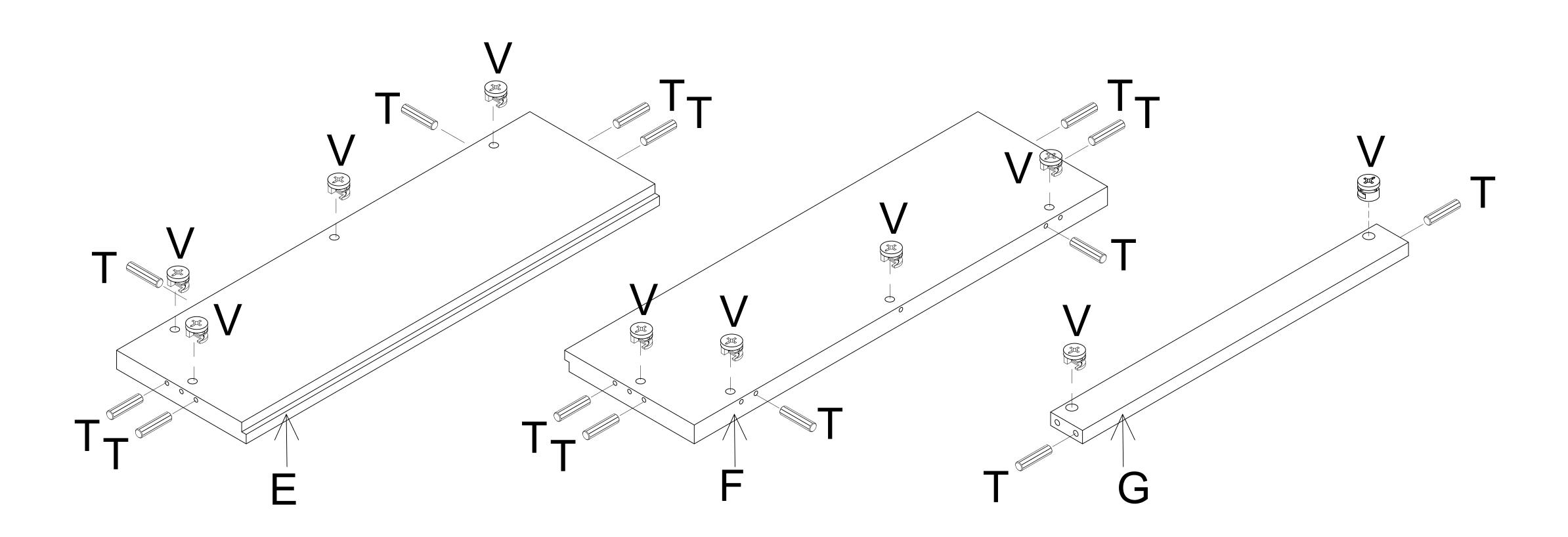
Attach the Left & Right Side Panel (B & C) to the Back Left & Right Panel (E & F), then attach the Center Bar (G) to the Left & Right Side Panel (B & C) and secure the Cam Lock (V) with a screwdriver (not provided). Cover the Cam Lock (V) with Cam Lock Cover (W).
