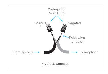
NOTE: THE SUBWOOFER CAN BE CONNECTED AT ANY POINT IN THE DAISY CHAIN.
