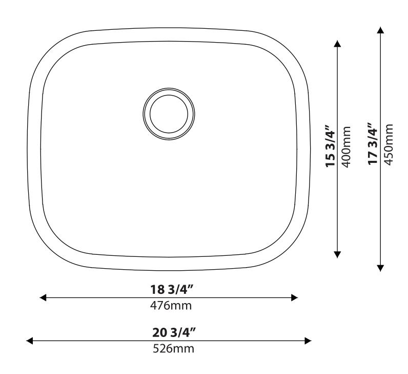
**NOTE:** Cutout template is provided as a guide **ONLY** and must be checked against actual sink to verify correct fit.
