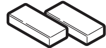
Filler blocks or scrap wood pieces, if needed for top cabinet spacing (used on recessed bottom cabinet installations only)
