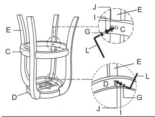
Take the Allen Wrench, and turn the bolts until the legs are secure. DO NOT TIGHTEN COMPLETELY. Stop when you feel you are adding force to tighten the bolt.
