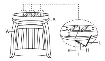
Keep the Backrest (A) and Cushion Seat (B) inverted on a stable raised surface. Attached the Swivel Plate located on the Apron With Swivel Plate (D) to the Cushion Seat (B) using Bolt (F), Lock Washer (I), Flat Washer (K) with Allen Wrench (L). Turn the Swivel Pub Stool right side up.
