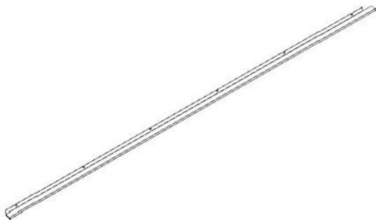
G01 CANALÓN - A4M03478 (x1) 1 \frac{9}{16}'' \times 1 \frac{15}{16}'' \times 1117 \frac{5}{16}'' (40 x 50 x 2838)
