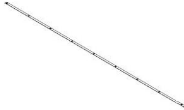
F01 BARRA PLANA - A4M02585 (x1) 1/16" x 1" x 110 3/4" (2 x 25 x 2813)
