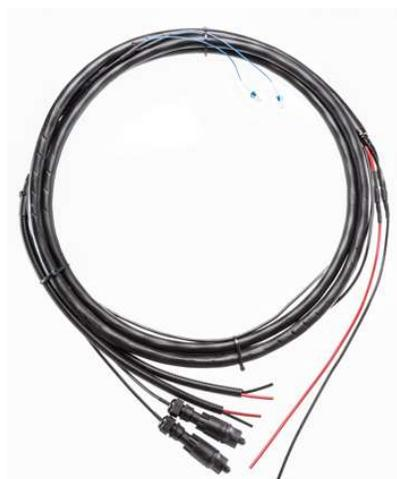
Y-SPLICE hybrid jumpers are designed for high-capacity dual band RRH's for macro application, 8AWG with 1 or 2 pair single mode optical fiber. They come with Duplex LC and FullAXS compatible connectors.
