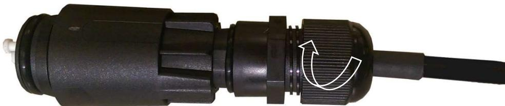
Engage the compression nut thread to the body 3-4 revolutions to keep the grommet in place but do not tighten fully to allow for adjustment during RRU connection.
