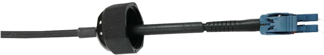
Carefully feed compression nut over fiber jumper connector and slide onto jacketing. Do not twist or bend the LC connector or fiber. Excessive force or bending may break the fiber or connector components.
