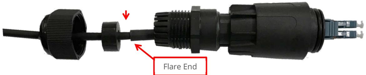
Wrap the rubber split grommet around the jacketing and **VERY CAREFULLY** push it **UNDER** the clamping fingers until the grommet is flush with the finger ends. **Caution: it will be necessary to gently lift the fingers.**
