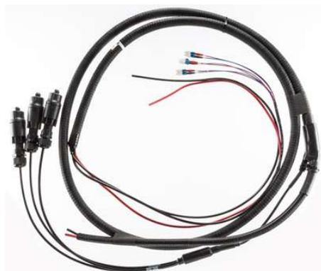
Hybrid jumpers for macro application, 1x1's or 1x2's, 8AWG with 1 to 4 pair single mode optical fiber. Designed to link junction box to RRH. All jumpers come Duplex LC, some with optional FullAXS compatible connectors, depending on model ordered. All jumpers are UL-Listed, flame-retardant jacket, UV protection, suitable in both indoor and outdoor applications.
