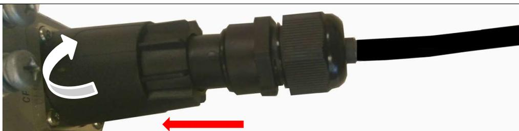
Slide the FullAXS compatible sleeve up to the RRH. Turn top nut clockwise to secure to RRH bulkhead connector.
