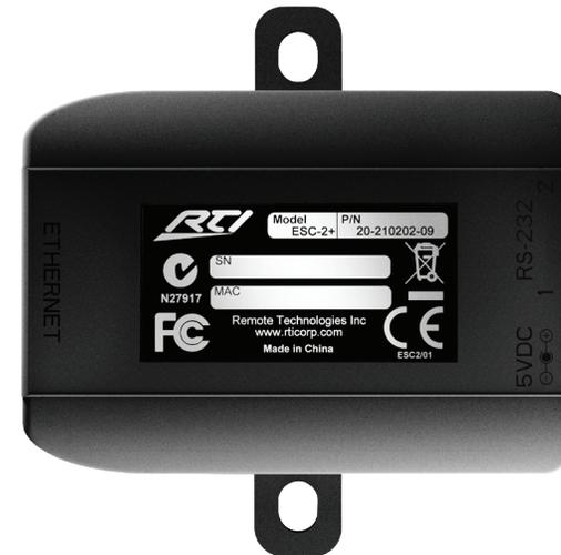
The ESC-2+ Ethernet to Serial Converter provides a convenient way to add two RS-232 ports with full two-way control capability to a system utilizing an RTI XP series control processor. Two built-in RJ-45 jacks and the included RJ-45 to DB9 adapters allow efficient cabling over standard Cat-5 wire between the ESC-2+ and the device being controlled. This allows full RS-232 control virtually anywhere there is access to an Ethernet network connection.
