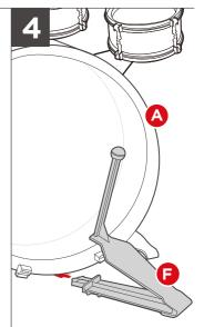
Insert the part F bass pedal into the mount at the bottom of the bass drum.
