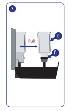
**To remove refill** Pull the container (e) and the pump housing (f). Please recycle accordingly.
