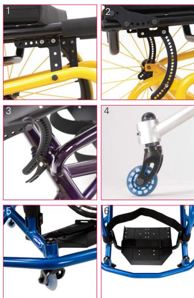
1. Front seat height and center-of-gravity adjustments
