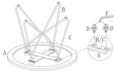
Attach the Leveler (G) to the Upper Leg (C) and Lower Leg (B).
