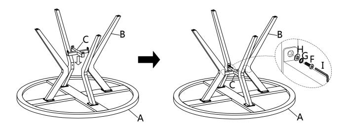
4 With assistance from your adult partners, turn the Dining Table right way up. Adjust the pre-installed levelers on the bottom of Leg (B) until the Dining Table is level with the ground.
