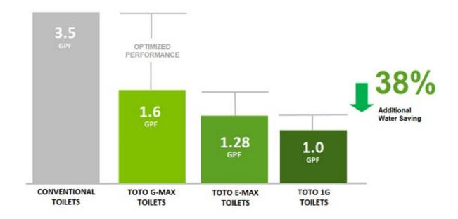
Utilizing the same proven engineering as our legendary 1.6 GPF G-Max flushing system, the 1.28 GPF E-Max and 1.0 GPF ultra-low flushing systems, such as Tornado Flush™ and Siphon Jet Flush, reinforce TOTO's performance reputation while offering an additional water savings of 20% and 38% respectively.
