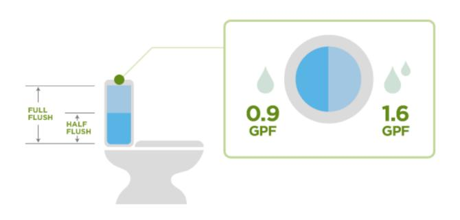
The dual flush system reduces water in the use phase.
