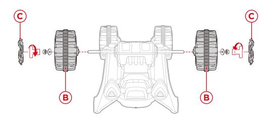
Remove the nuts/washers from the front axle. Slide a washer and part B wheel onto the axle, then replace the nut/washer to secure the wheel. Repeat on the other side. Snap a part C hub cap on each wheel.
