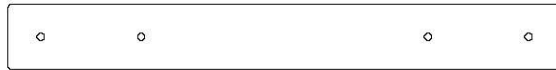
M4 | LATTE MURALE - W4L16098 (x2) | 5/8 po x 3 3/8 po x 28 7/8 po (16 x 86 x 734)
