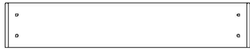
M8 RAIL MURAL - W4L04466 (x1) 5/8 po x 3 3/8 po x 18 3/4 po (16 x 86 x 475)
