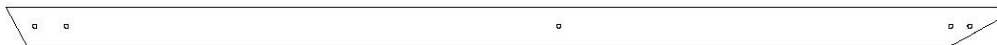
E51 | CALE ANGULAIRE - W4L16004 (x2) | 1 7/16 po x 3 3/8 po x 87 3/16 po (36 x 86 x 2214)
