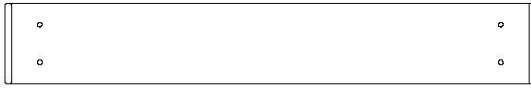
M5 RAIL MURAL - W4L04465 (x1) 5/8 po x 3 3/8 po x 22 po (16 x 86 x 563)
