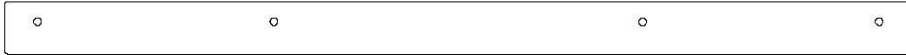
H4 | SUPPORT DE PLANCHER - W4L04470 (x1) | 1 po x 2 3/4 po x 47 3/8 po (24 x 70 x 1204)
