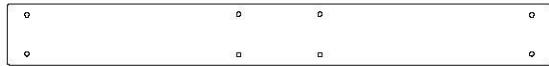
G1 | RAIL DE LA BALANÇOIRE - W4L04483 (x1) | 1 po x 5 1/4 po x 47 3/8 po (24 x 134 x 1204)
