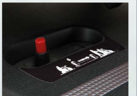
Two-step disengaging lever to help prevent free-wheeling
