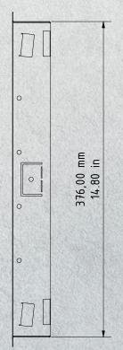
General tolerance DIN/EN 2768 -mK Wall cut-out dimension +4 mm/0.15 in
