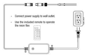
Note: When using outdoors, plug the unit into an appropriately rated GFCI receptacle with cover.
