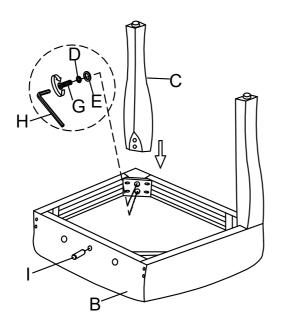
Take the Allen Key, and turn the bolts until the legs are secure. DO NOT TIGHTEN COMPLETELY. Stop when you feel you are adding force to tighten the bolt.
