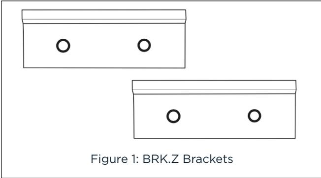
2. After choosing an installation area (securing brackets to wall studs is recommended), level and mark both bracket heights, so they are level to each other.
