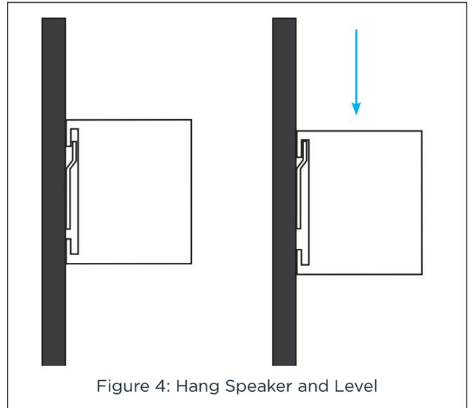
5. If the speaker is at an acceptable height/level, then wire and hang the speaker and attach the grille to complete the installation.
