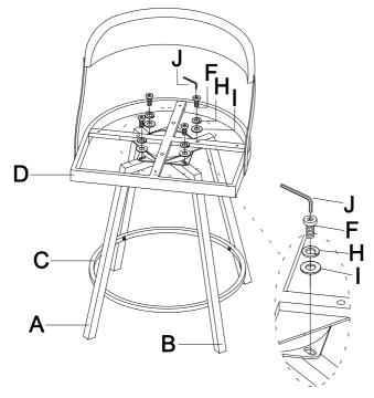
Stand the chair on an even surface and check for balance. If the chair wobbles slightly, apply downward pressure on the uneven leg and tighten the bolts to correct the imbalance. Once the chair is balanced, apply downward pressure evenly in the center of the chair and tighten all bolts, being careful not to over-tighten beyond the hole depth.
