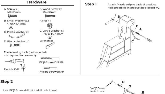
Do not drill an oversized hole or the wall anchor will not hold tightly into the wall.
