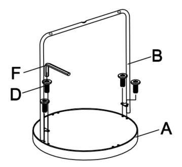
Attach Under Side Panel (C) to Wood Top (A) by Bolt (D) and Allen Wrench (F). Then attach two side panels together by Bolt (E) and Allen Wrench (F) as shown.
