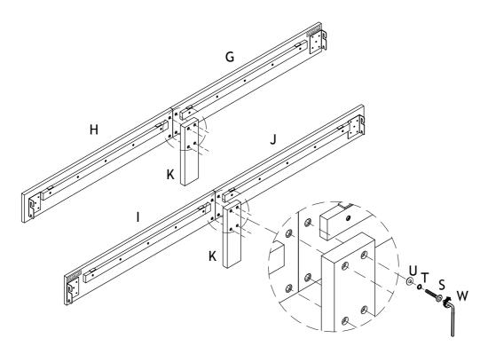
Attach Left Side Rail - Front & Rear (G & H) and Right Side Rail - Front & Rear (I & J) to Headboard Leg - Left & Right (B & C) and Footboard Leg - Left & Right (E & F) and tighten JCBB Bolt (P) and Flat Washer (R) with Allen Key (V).
