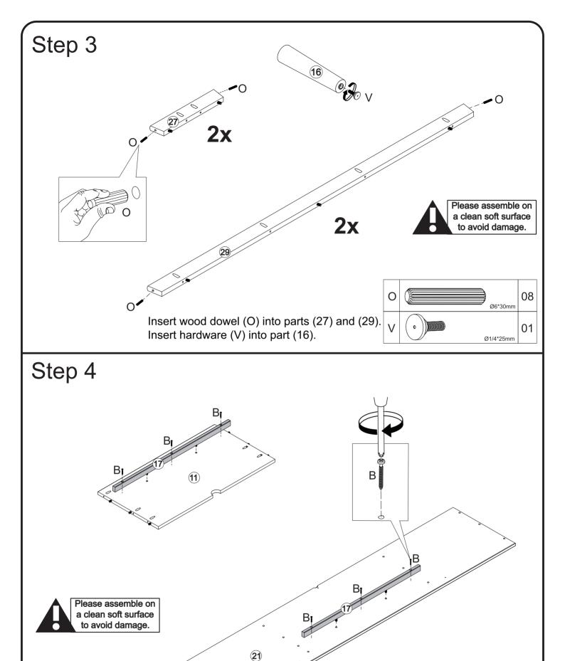
Attach parts (17) to parts (11) and (21) with
