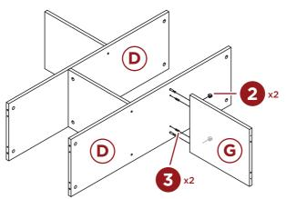
Insert eight part 2 cam locks into the two part D middle shelves, four locks per shelf. Insert eight part 3 dowels into the two part C side panels, four dowels per side.
