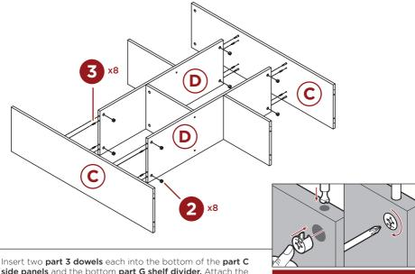
side panels and the bottom part G shelf divider. Attach the part B shelf bottom with six part 4 screws.
