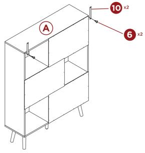
Place the assembled product in its intended space, abutting a wall. Stretch the straps to sit flat against the wall, then use a pencil to mark the wall, use the strap's pilot hole as a guide.
