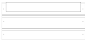
WP6 | CLOISON CENTRALE SUPÉRIEURE - W2A02979 (x2) 1 1/2"x9 3/4"x20 7/8" (38x248x530)
