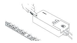
2. Each time a new Receiver is set up for the first time, clear the memory by pressing and holding the "Learn" button until the lights blink.
