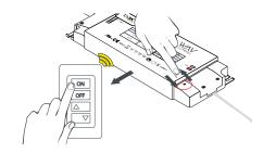
3. Very quickly, click and release the "Prog" button and, within 5 seconds, quickly click and release the "Up Arrow" button on the Controller for any of the Zones. When lights blink, Controller and WAV Smart Receiver are paired.
