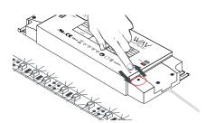
2. Each time a new WAV Smart Receiver is set up for the first time, clear the memory by pressing and holding the "Prog" button until the lights blink.
