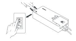
3. Very quickly, click and release the "Prog" button and, within 5 seconds, quickly click and release the "Up Arrow" button on the Controller for any of the Zones. When lights blink, Controller and WAV Smart Receiver are paired.
