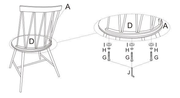
Stand the chair on an even surface and check for balance. If the chair wobbles slightly, apply downward pressure on the uneven leg and tighten the bolts to correct the imbalance. Once the chair is balanced, apply downward pressure evenly in the center of the chair and tighten all bolts, being careful not to over-tighten beyond the hole depth.
