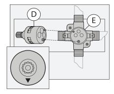
4) Align spindle extender (C) with broach on cartridge (D). Install spindle extender (C) and cap assembly (A) to cartridge (D). Secure cap assembly (A) by turning clockwise.
