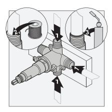
**Optional:** Apply plumber tape to male IPS threads on the inlet and outlet ports of diverter valve. Install 1/2"-14 NPT copper fittings to the inlet and outlet ports. Connect outlets to desired accessories.
