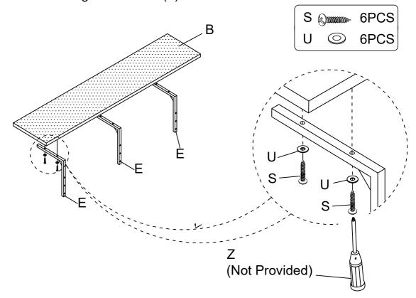
Assemble Shelf Support Tube (E) to the Desk Top Board (A) with Bolt (P), Flat Washer (U), then fastened using Screwdriver (Z).
