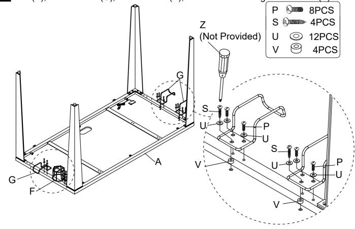
Assemble Keyboard Bracket (K) to the Desk Top Board (A) with Bolt (P), Flat Washer (U), then fastened using Screwdriver (Z).
