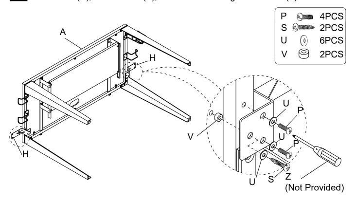
Assemble Tray Board (I) to the Support Bracket (H) with Bolt (Q), Flat Washer (U), then fastened using Screwdriver (Z).
