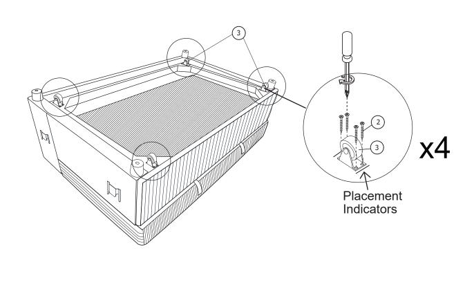
STEP 3: Attach Back (B) to Base (A) by aligning the metal brackets and pushing down until securely attached.
