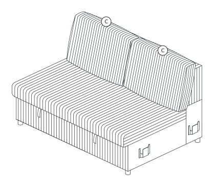
STEP 5: Align the sectional upholstery and connect them together by sliding the metal hooks into place until secure.
