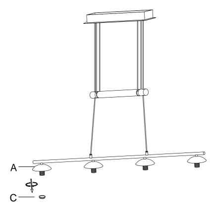
Assemble the Lamp Shade (B) to Lamp Body (A) and using the Ring (C) to tight it. Then, assemble the Bulb (I) to the lamp holder in the Lamp Shade (B).
