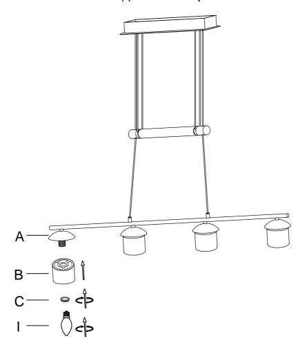
Firstly, remove Bolt (H) from the ceiling base of Lamp Body (A) and take out the bracket. Secondly, use Bolt (E) and Flat Washer (D) to tight the bracket on the ceiling by screwdriver, connect Wire Connector (F) & Wire Connector (G) together with cable. Finally, put the ceiling base back to cover the bracket and using Bolt (H) by screwdriver to fix them.
