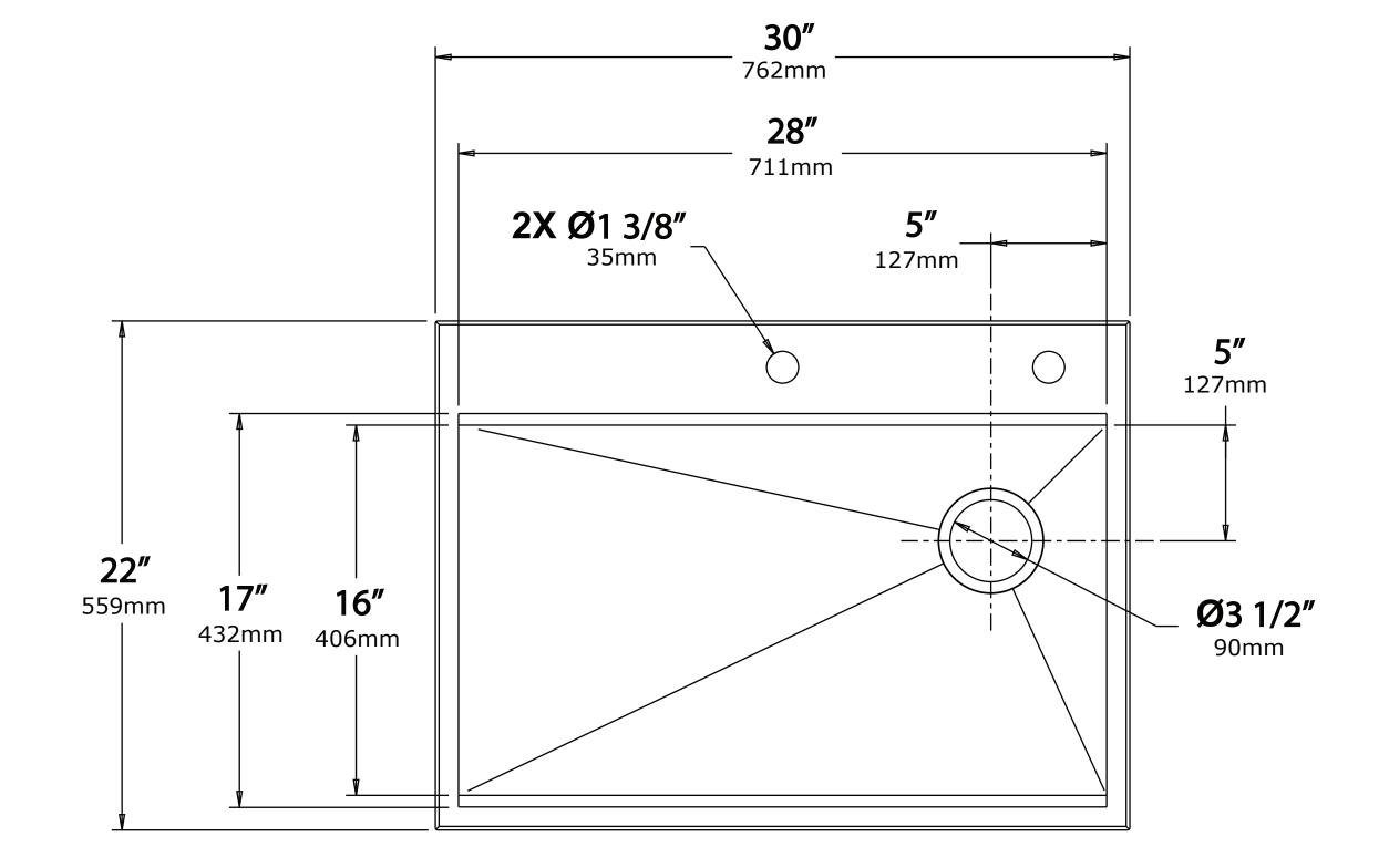
**NOTE:** Cutout template is provided as a guide **ONLY** and must be checked against actual sink to verify correct fit.
