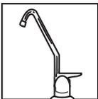
**Run water through faucet for three minutes on single systems and seven on dual systems to purge cartridge of air.**
