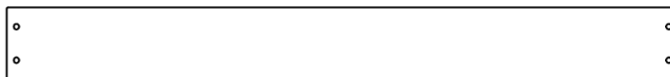
K02 | TABLA DE LA BASE/CAJA DE ARENA - W4L16035 (x3) | 5/8"x5 1/4"x49" (16x134x1244)
