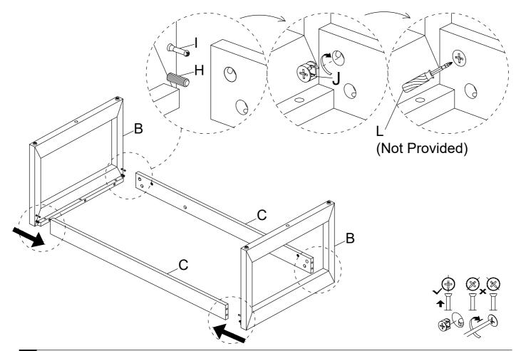
4 Attach the Side Panel (C) and Side Frame (B) to Top Panel (A), then secure Cam Lock Screw (I) with Cam Lock Nut (J) by Screwdriver (L).
