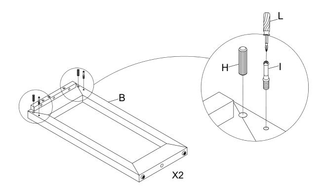
2 Insert the Wood Dowel (H) and Cam Lock Screw (I) to the Top Panel (A), then secure Cam Lock Screw (I) by Screwdriver (L).
