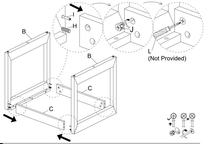
4 Attach the Side Panel (C) and Side Frame (B) to Top Panel (A), then secure Cam Lock Screw (I) with Cam Lock Nut (J) by Screwdriver (L).
