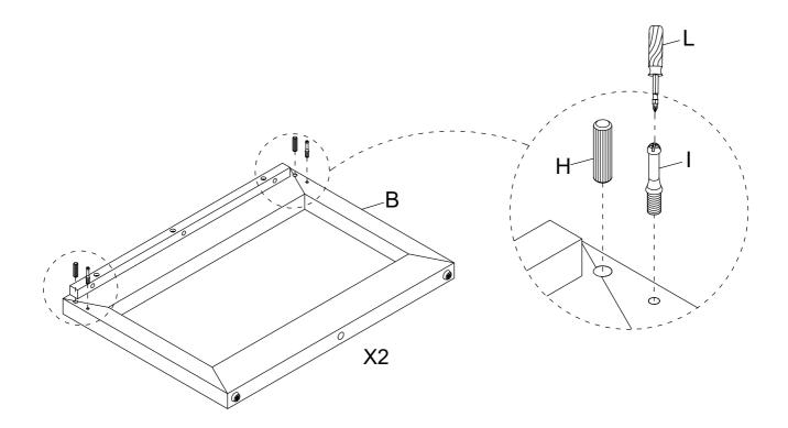
2 Insert the Wood Dowel (H) and Cam Lock Screw (I) to the Top Panel (A), then secure Cam Lock Screw (I) by Screwdriver (L).
