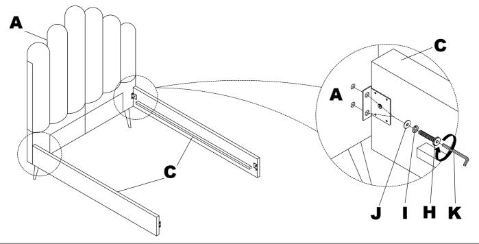
Attach Side Rail (C) to Footboard (B) by using Allen Bolt (H), Spring Washer (I) and Flat Washer (J) and tightening with Allen Key (K).
