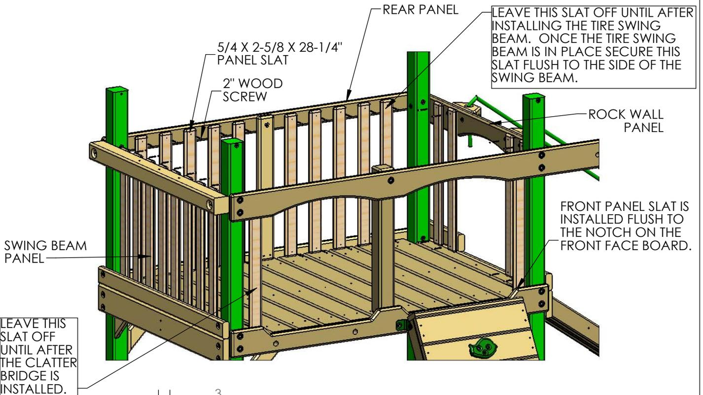
LEAVE THIS SLAT OFF UNTIL AFTER THE CLATTER BRIDGE IS INSTALLED.
