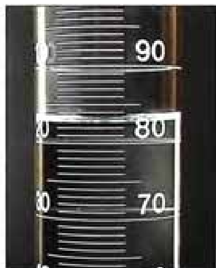
Figure 1.6. Reading the significant digits on a graduated cylinder.
