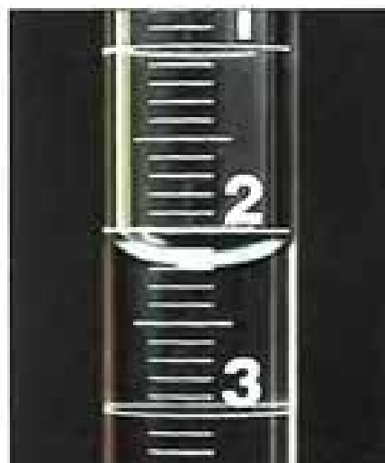
Figure 1.5. Reading the significant digits on a buret.
