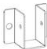
J18 PERGOLA BRACKET - A4M05292 (x28) 4 7/16"x2 1/16"x3 5/8" (88x53x112)
