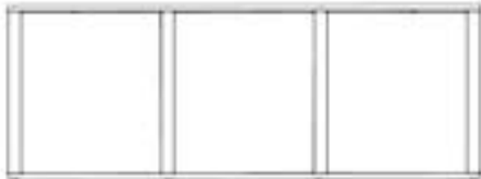
E01 PURLIN FRAME - A4M05032 (x4) 13/16"x21 5/16" 56 1/2" (21x541x1435)
