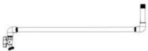
WATER LINE ASSEMBLY FROM STEP 179
