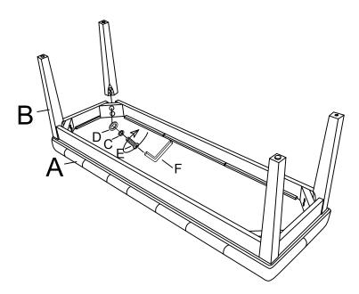
Stand chair up on an even surface and check that it is balanced. If there is a slight wobble, apply downward pressure in the corner where a leg is uneven. Keeping pressure in that corner, tighten all bolts.
