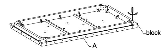
Upside down the table top(A), attach 4pcs legs(B) and install use bolt(D), lock washer(E) and flat washer(F), tight by allen wrench(C).
