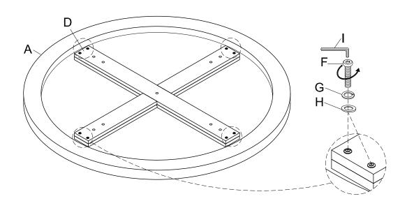
Attach the Mounting Rail (D) to the top of the Upper & Lower Leg (B & C) using Short Bolt (F), Lock Washer (G) and Flat Wahser (H) with the Allen Key (I).
