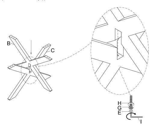
Remove the Mounting Rail (D), Short Bolt (F), Lock Washer (G) and Flat Wahser (H) from the bottom of the Table Top (A) with the Allen Key (I).
