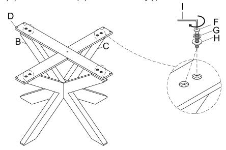
Attach the assembled base to the bottom of the Table Top (A) using Short Bolt (F), Lock Washer (G) and Flat Washer (H) with the Allen Key (I).
