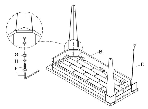
2 First, assemble Bottom Panel (C) to Leg (D), using Bolt (E), Lock Washer (H) and Flat Washer (G) by Allen Key (I). Second, assemble the last Leg (D) to Top Frame (B) & Bottom Panel (C), using Bolt (F), Bolt (E), Lock Washer (H) and Flat Washer (G) by Allen Key (I) as below shown.
