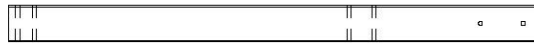
SP01 | SUPPORT DE POUTRE DE BALANÇOIRE - W4L16462 (x1) 3 3/8 po x 3 3/8 po x 50 po (86x86x1269)
