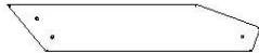
H12 | PLANCHE DU PIGNON - W4L15988 (x4) | 1 po x 3 3/8 po x 18 1/4 po (24x86x465)
