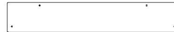
K05 | PLANCHE DE PLANCHER - W4L15979 (x1) | 5/8 po x 4 3/4 po x 27 5/8 po (16x120x701)
