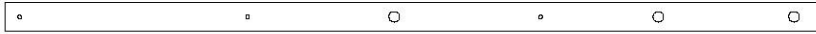
B09 | PLANCHE DE CORDE - W4L15740 (x1) | 3 po x 3 po x 85 3/8 po (76x76x2170)
