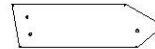
H13 | PLANCHE DU PIGNON - W4L15989 (x4) | 1 po x 3 3/8 po x 11 3/4 po (24x86x300)
