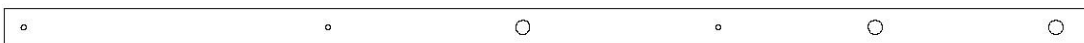
B09 | PLANCHE DE CORDE - W4L15740 (x1) | 3 po x 3 po x 85 3/8 po (76x76x2170)
