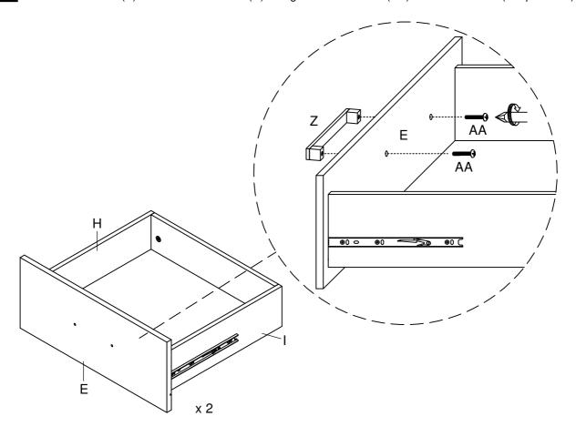
20 Slide out the bearing and align the position then push the 2 pieces drawers to inside exactly by your hand as shown.
