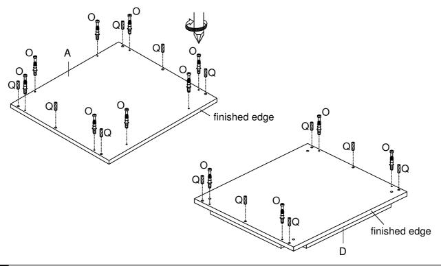
2 Insert Minifix Cam Lock (P) and Wood Dowel (Q) to the Top & Center Support Rail (K & L) as shown.
