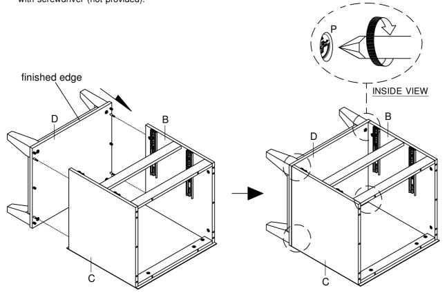
9 Attach the Top Panel (A) to the Left & Right Side Panel (B & C) and Top Support Rail (K) and tighten the Minifix Cam Lock (P) with screwdriver (not provided).
