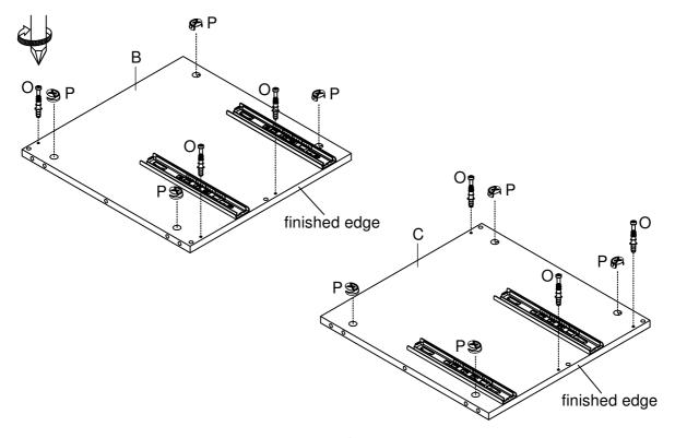
5 Attach the Top Support Rail (K) and Center Support Rail (L) to the Left Side Panel (B) and tighten the Minifix Cam Lock (P) with screwdriver (not provided).
