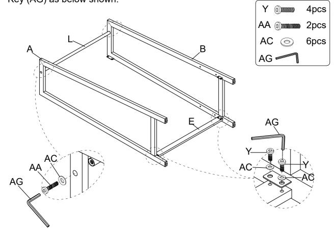
Assemble Back Panel - Top (C) & Front Panel - Bottom (E) to Left Frame (A) and Right Frame (B), using Bolt (Y), Flat Washer (AC) and the iron sheet of Anti-Tipping Kit (AH) to tighten by Allen Key (AG) as below shown.
