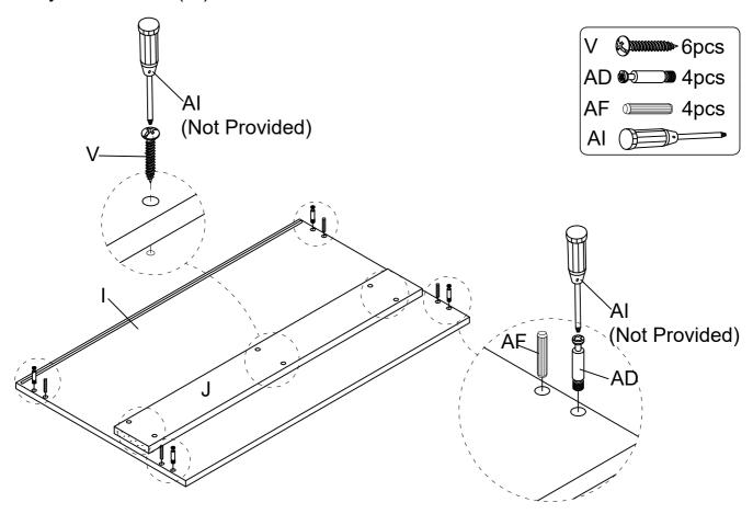
Assemble Top Panel (I) to Left Panel (F) and Right Panel (G), using Nut (AE) to lock with Bolt (AD) & Wood Dowel (AF) by Screwdriver (AI).
