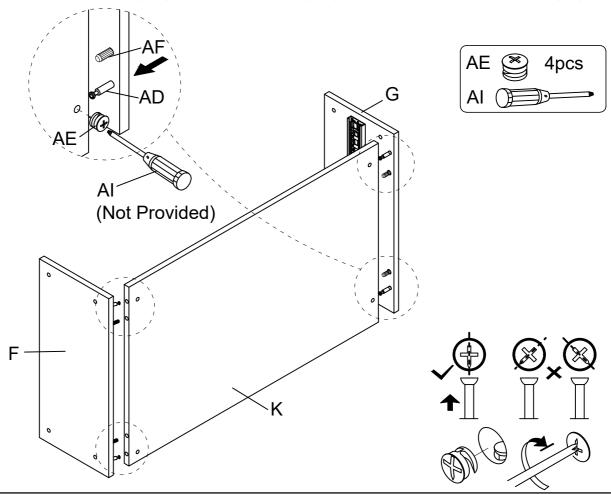
Put Back Panel (H) into Left Panel (F), Right Panel (G) and Bottom Panel (K) as below shown.
