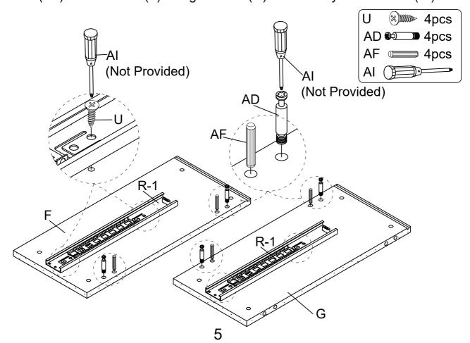
Assemble Bottom Panel (K) to Left Panel (F) and Right Panel (G), using Nut (AE) to lock with Bolt (AD) & Wood Dowel (AF) to tighten by Screwdriver (AI).
