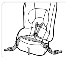
Finished Lower Anchor Belt Routing
