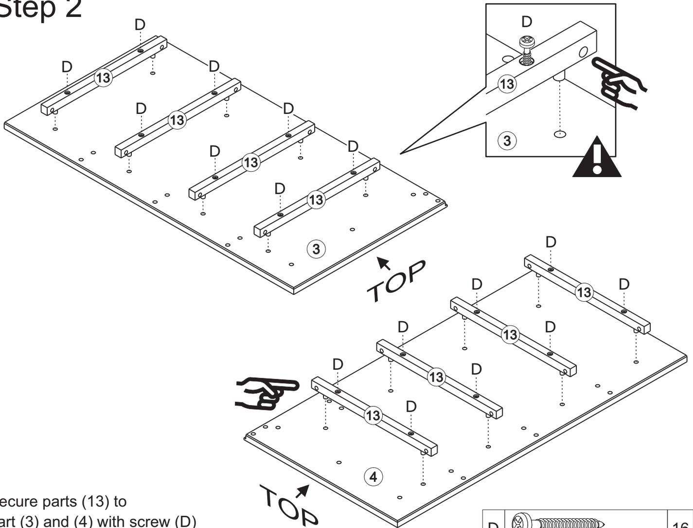
Secure parts (13) to part (3) and (4) with screw (D) and screwdriver (not included).
