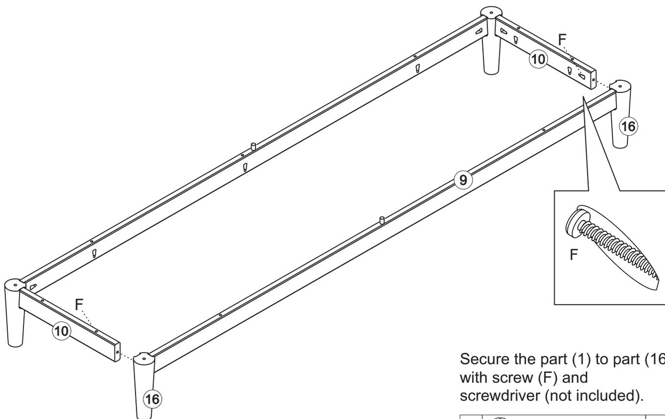
Secure the part (1) to part (16), with screw (F) and screwdriver (not included).
