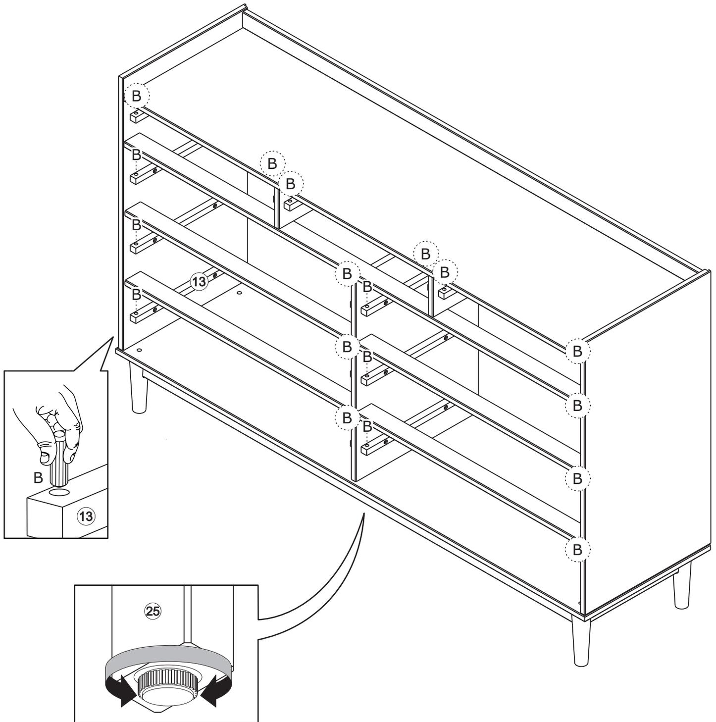
Insert wooden dowel (B) into part (13) to be the stop of the drawer.
