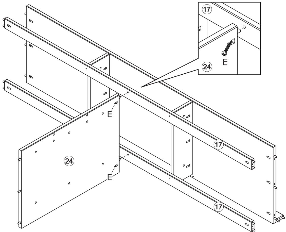
Secure part (24) to parts (17) with screw (E) and screwdriver (not included).
