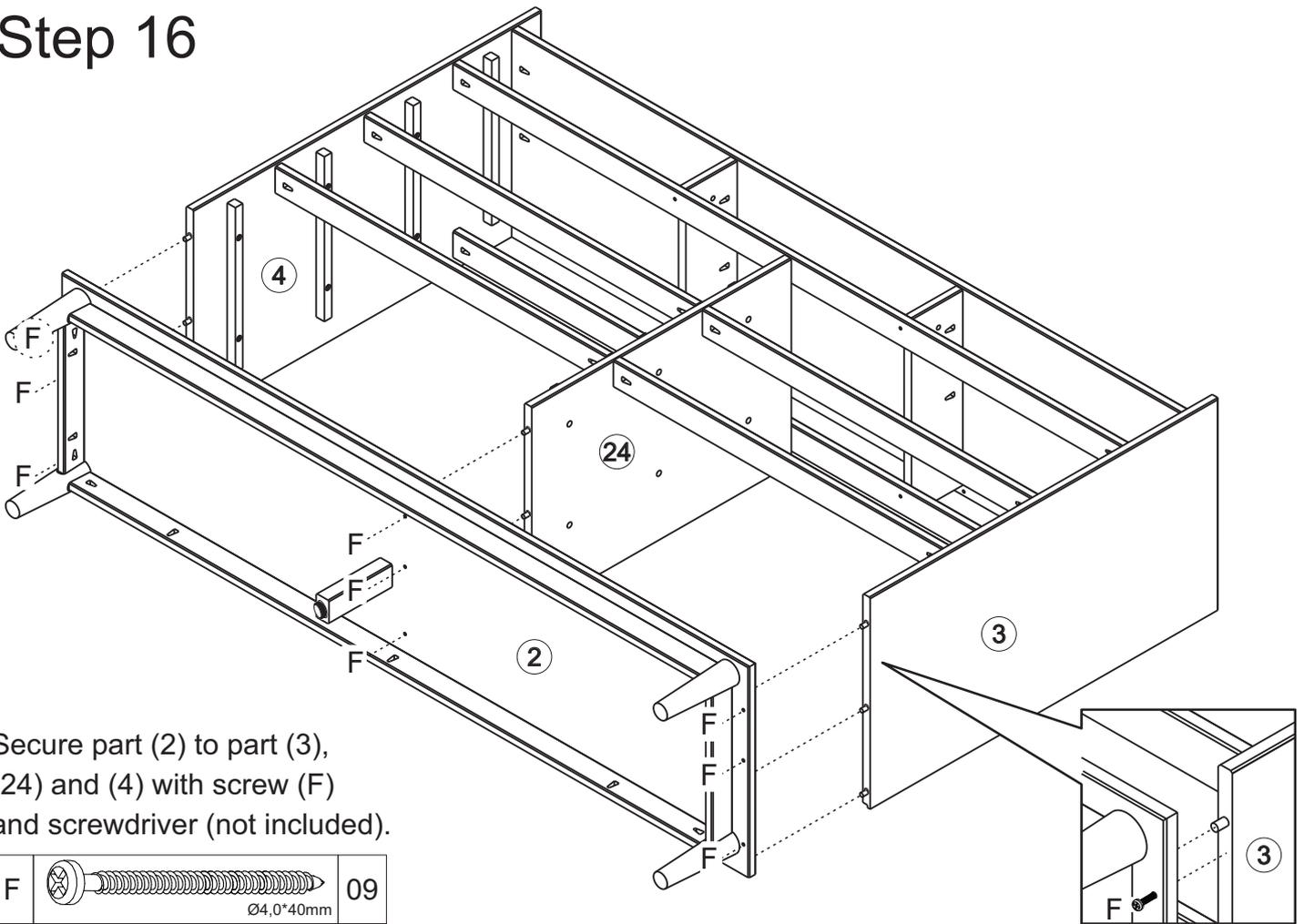
Secure part (2) to part (3), (24) and (4) with screw (F) and screwdriver (not included).
