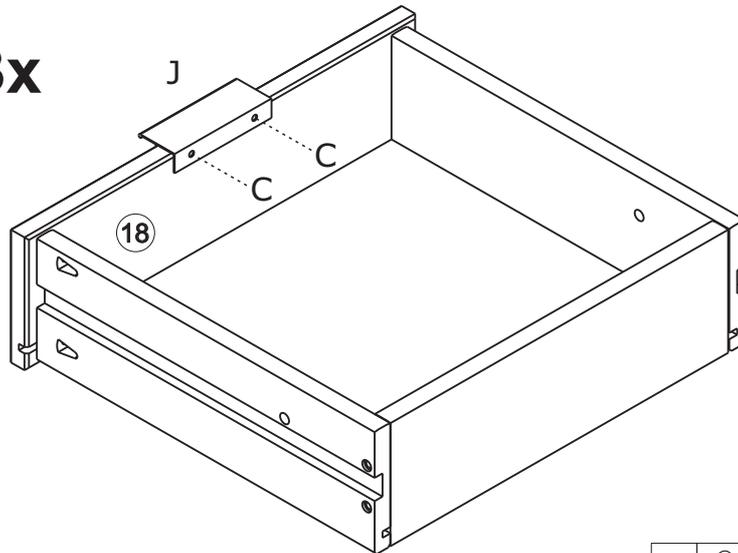
Secure handle (J) with screw (C) and screwdriver (not included), in the pre holes on the drawer front.
