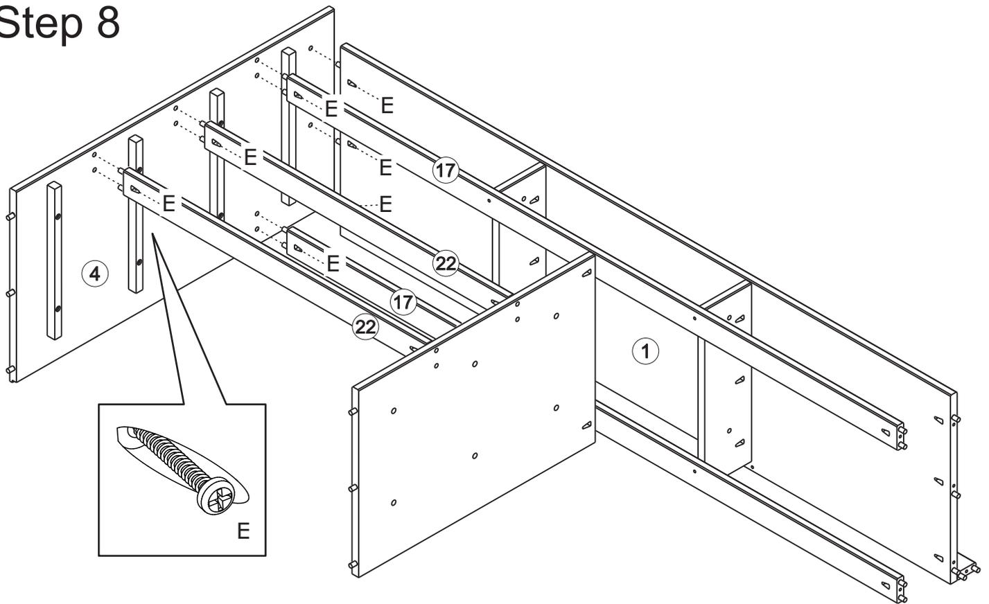
Secure parts (1), (17), and (22) to part (4) with screw (E) and screwdriver (not included).
