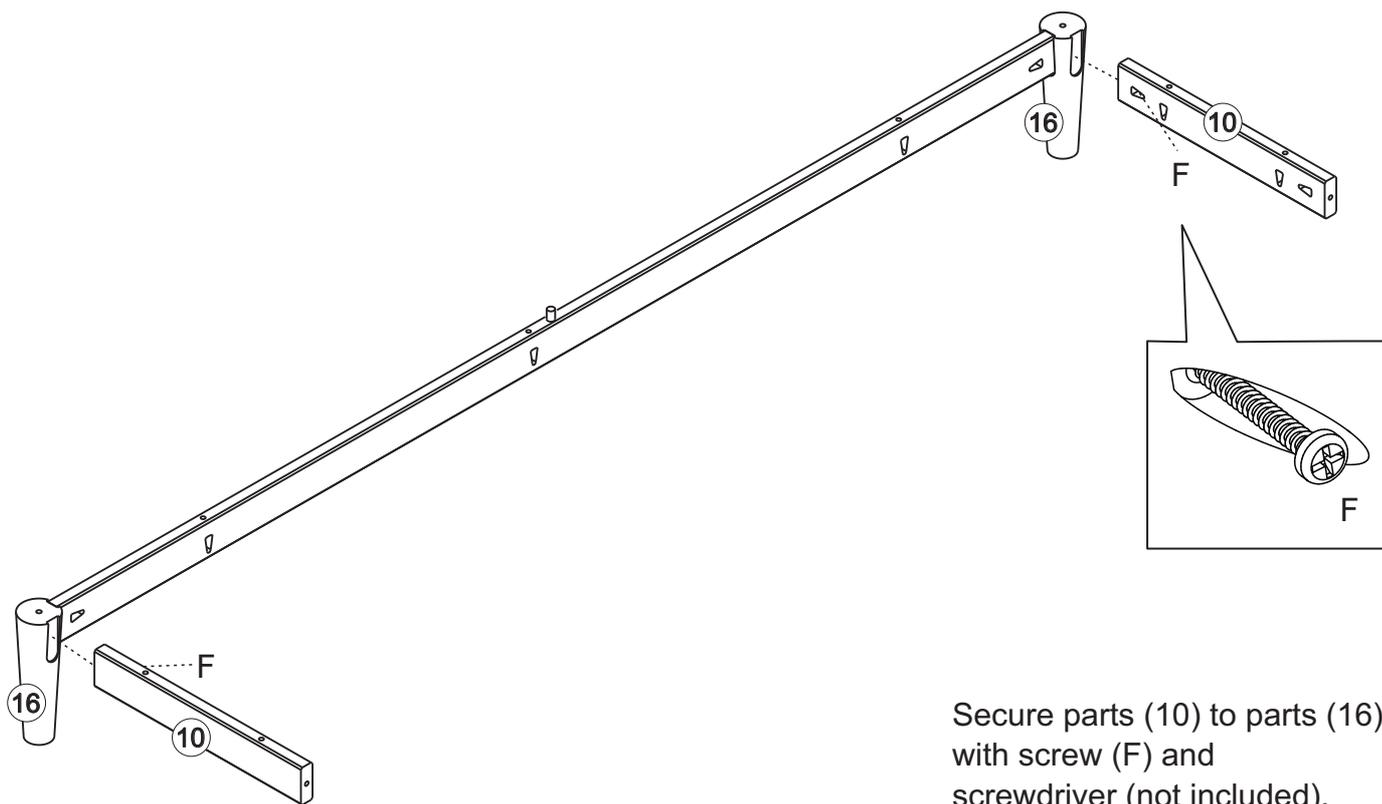
Secure parts (10) to parts (16), with screw (F) and screwdriver (not included).
