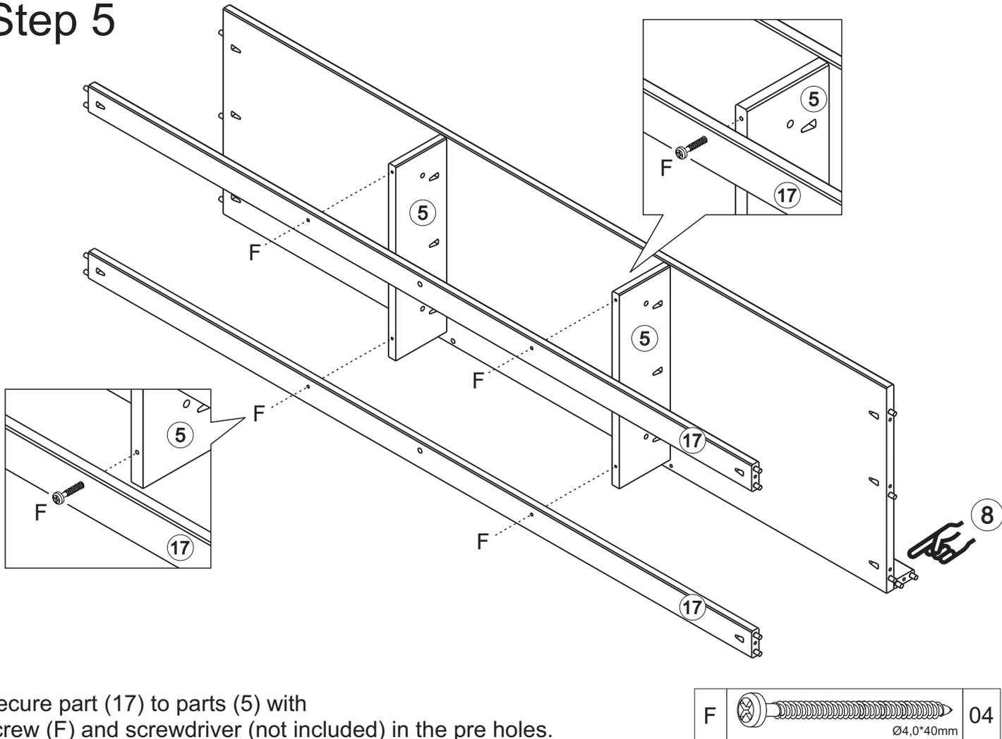
Secure part (17) to parts (5) with screw (F) and screwdriver (not included) in the pre holes.
