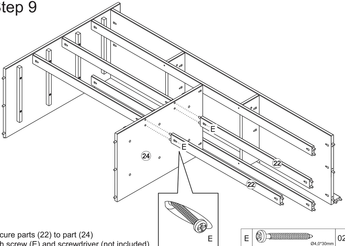
Secure parts (22) to part (24) with screw (E) and screwdriver (not included).
