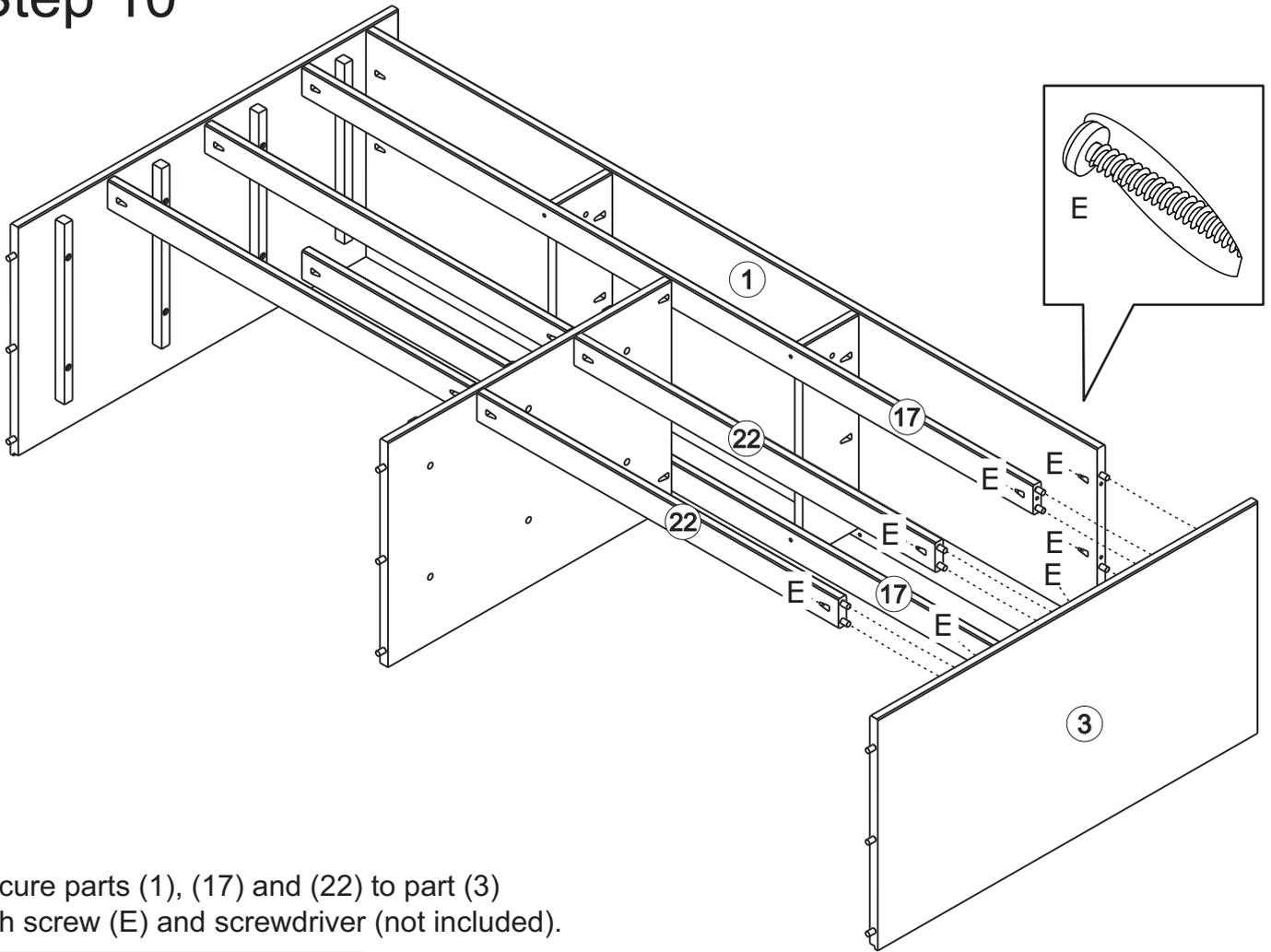
Secure parts (1), (17) and (22) to part (3) with screw (E) and screwdriver (not included).
