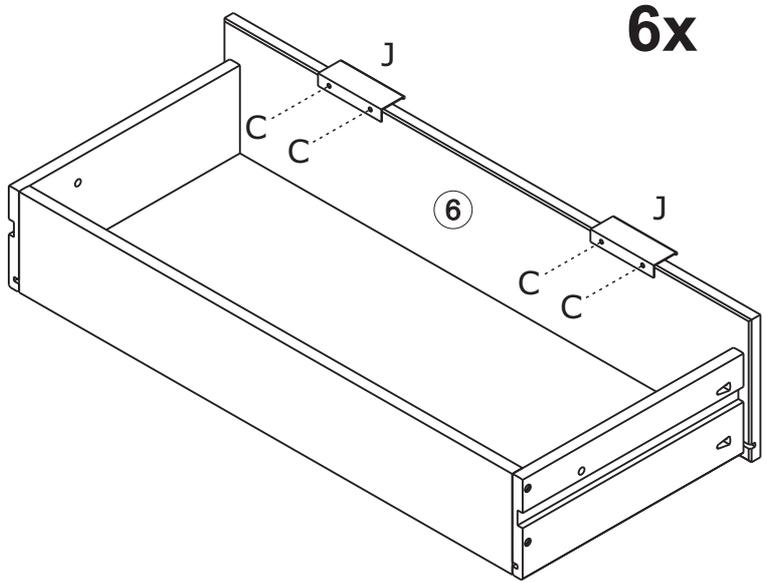
Secure handle (J) with screw (C) and screwdriver (not included), in the pre holes on the drawer front.
