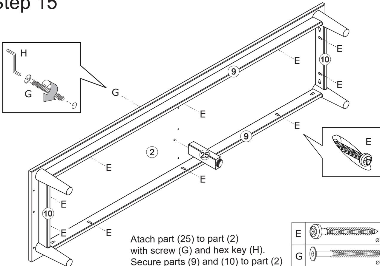
Attach part (25) to part (2) with screw (G) and hex key (H). Secure parts (9) and (10) to part (2) and attach with screw (E) and screwdriver (not included).
