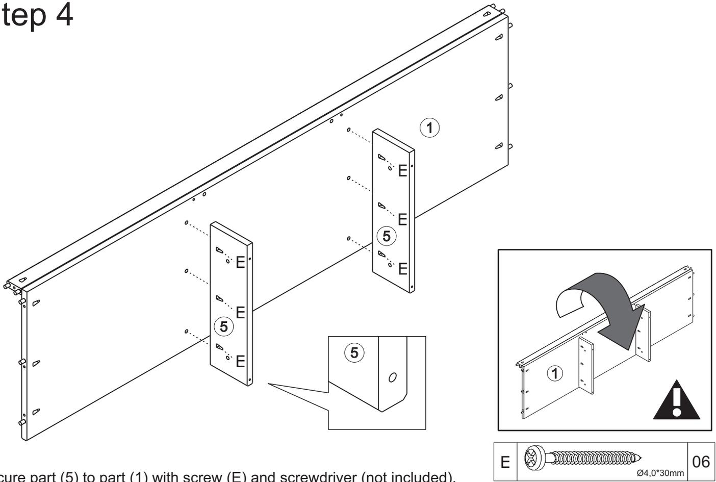
Secure part (5) to part (1) with screw (E) and screwdriver (not included).
