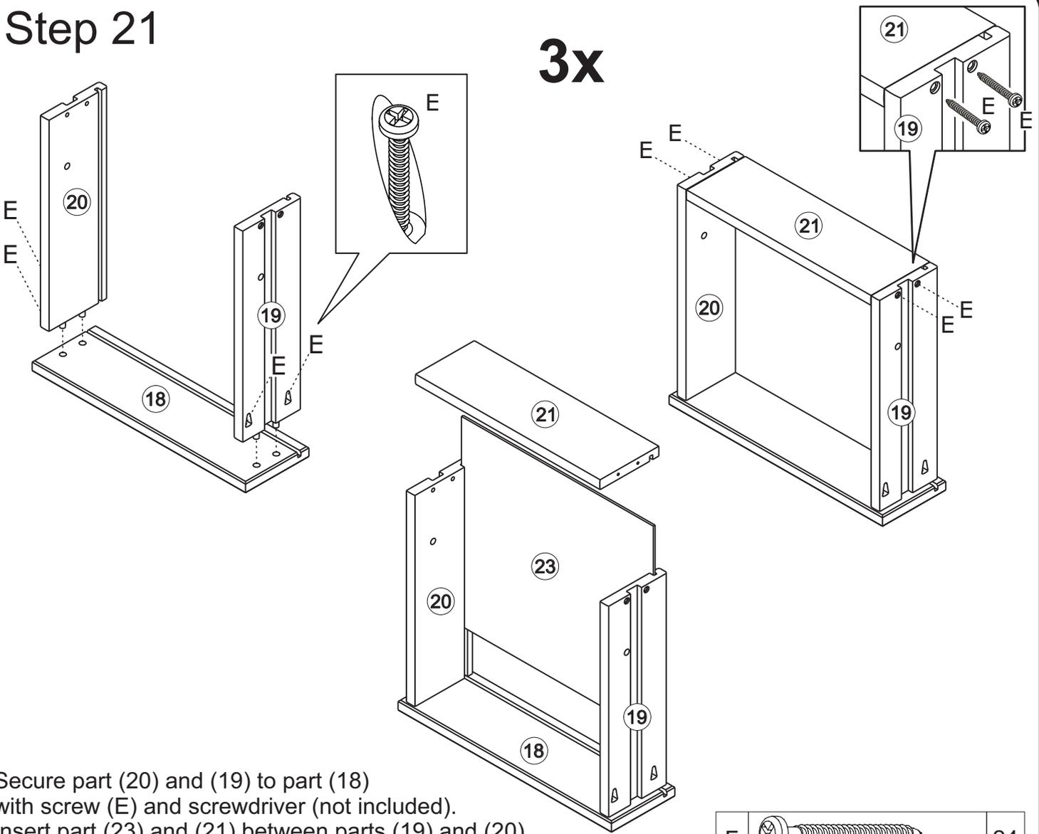
Secure part (20) and (19) to part (18) with screw (E) and screwdriver (not included).
