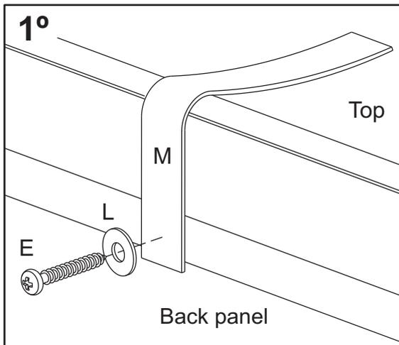
Drill your wall with a 6mm drill (not included) and insert hardware (K), securing wall anchor (M) into washer (L) and screw (E) in the wall.
