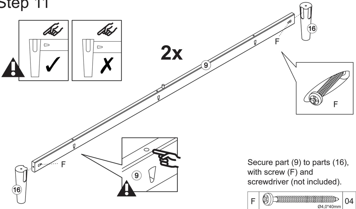
Secure part (9) to parts (16), with screw (F) and screwdriver (not included).
