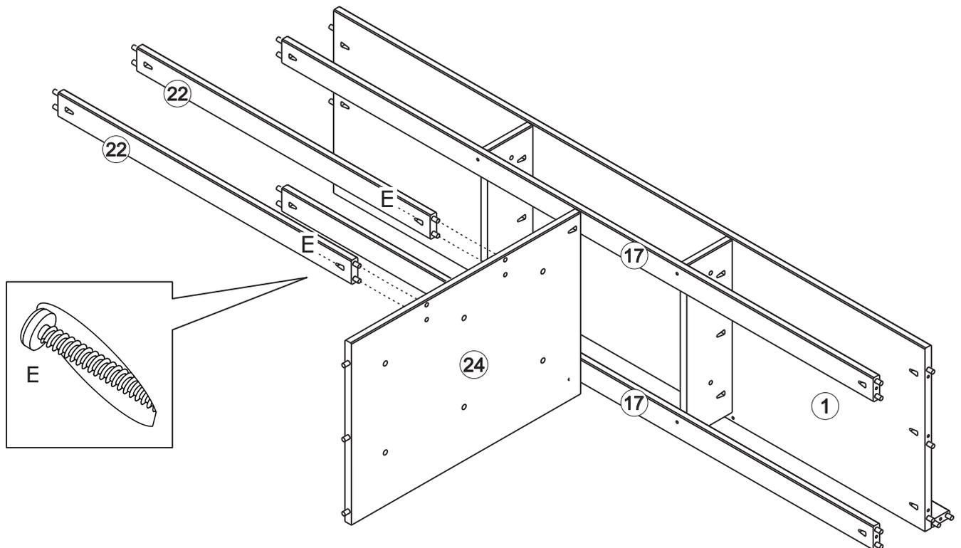
Secure parts (22) to part (24) with screw (E) and screwdriver (not included).
